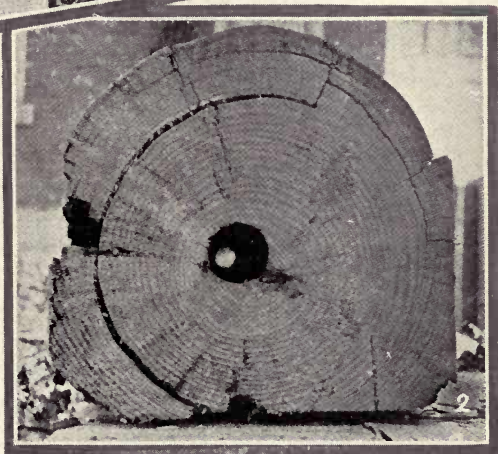
1.—A fungus plant that has eaten away the end of a mill beam
